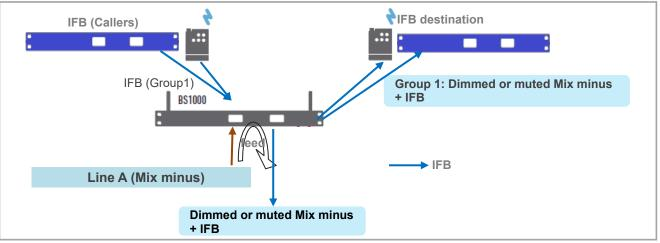
For information for the IFB settings on the BS1000, refer the BS1000 settings in the GCMW User Manual. In the BS1000 settings, if you select the Line Feed and a Genie group channel that applies the IFB, the FB audio (Mute or dimmed) and Genie group channel are mixed and output to the Line.
