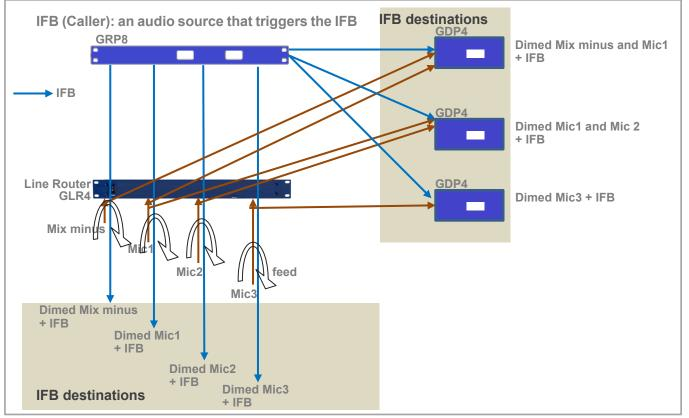
By setting the Talk key on the IFB destination, you can do different types of IFB configurations. Line input audio from the Line Router GLR4 can be sent back to the Line output. Even so, IFB dim level applies to the Line output audio.
