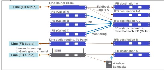
The input/output audio on the GLR4 Line can be connected to all IFB destinations and Genie group channels. FB audio can be transferred directly to the Genie group channel by connecting to the Base Station BS1000 (or BS850). If you are using a Line connection to BS1000, the IFB dim level applies to Genie group channels, so you can use the wireless Beltpack BP850 as an IFB receiver.
